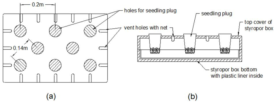
Figure 1: Detail of growing box (a – top view; b – side cross-section).
